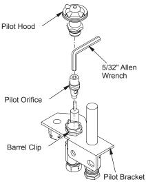
Figure 10 - Converting Pilot Orifice
